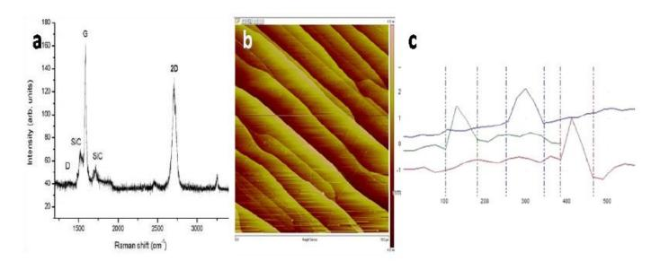
We tested the products by AFM and Raman. The G peak value is 1580cm<sup>-1</sup> and the 2D peak value is 2700cm<sup>-1</sup>, the 2D peak is sharp and symmetrical, and it has the characteristic of Lorentzien peak type. The half width of the 2D peak is 56 cm<sup>-1</sup> and 70 cm<sup>-1</sup>. AFM results show that the surface morphology of graphene is good, the thickness is 0.77 nm.
